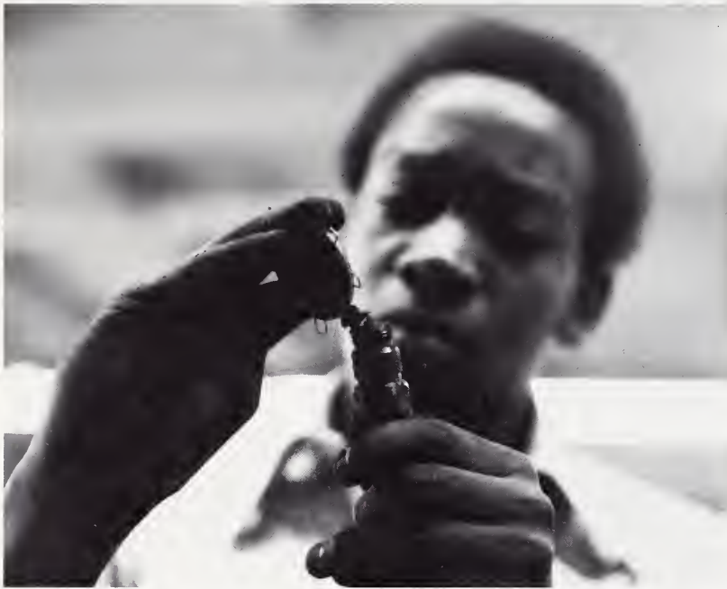
STEVE THOMAS Checks "gap" in a spark plug.
